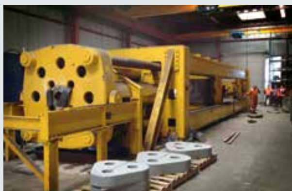
Pull and push testbed 16,000 kN
